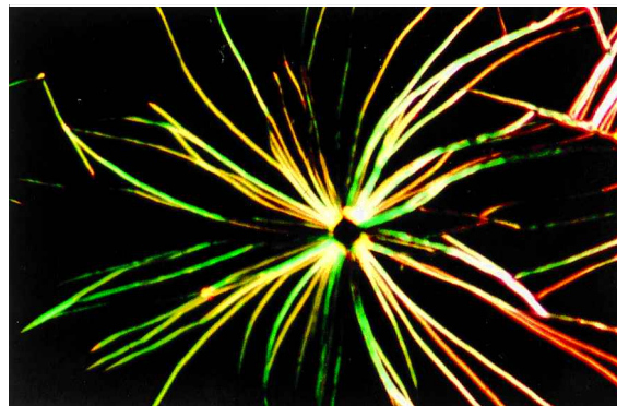
Figure 5. Vermis texture of the TGB phase of KI-5T at 145°C (no surface treatment).
